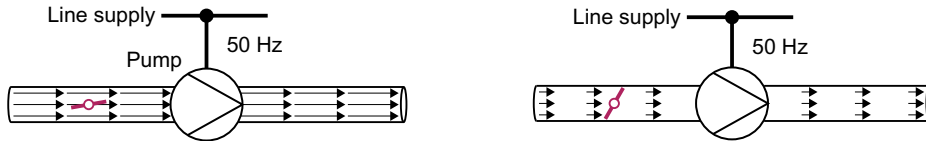
Figure 8-212 Flow control with pump and throttle connected to a 50 Hz line supply
