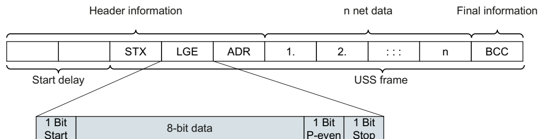
Figure 8-35 Structure of a USS telegram
