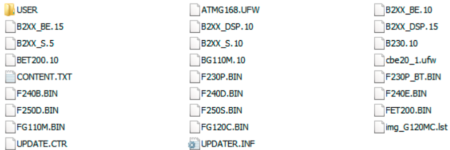
Figure 11-2 Example of memory card contents after the file transfer
